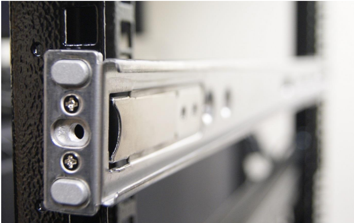
Figure 2-5: Front of outer rail correctly installed
