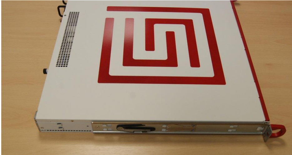
Figure 2-3: Pre-installed inner rail
